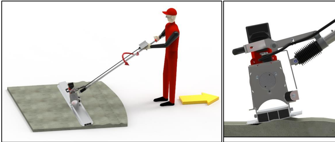
Figure 12: Schematic diagram of backwards concrete finishing with the HAL200Li.
